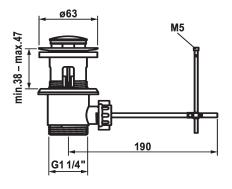
\* with long drainage slots \* also suitable for thin-walled sinks
