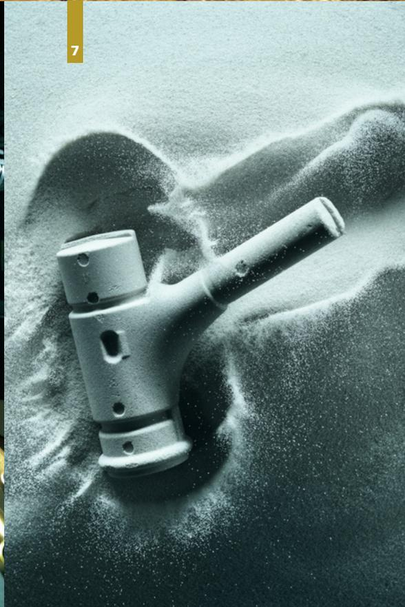
**5** — To make the fittings, pure brass, which arrives in the form of ingots, is used. **6** — The basic shape of the fitting in brass. **7** — With low-pressure die casting, the brass is first melted and then poured into sand molds, creating the basic shape of the fitting in brass.
